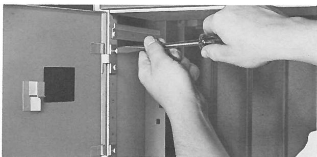
Fig. 20 Assembly of Hinges and Guides
