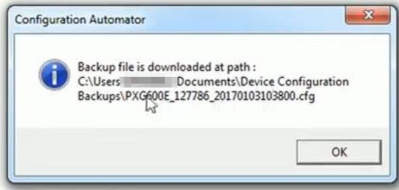
This file can be restored to the PXG, but must be done using the PXG web interface, not this loader (this program only supports XML formats and this backup file is a different format)
