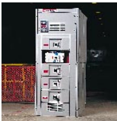
Five L- or N-frame breakers with Digitrip OPTIM Trip Units and one Breaker Interface Module can be mounted in a single 36-inch (914.40-mm) wide distribution structure. Six L- or N-frame breakers can be mounted when the Breaker Interface Module is mounted in another section or is not required.
