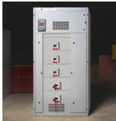
Five L- or N-frame breakers with Digitrip OPTIM Trip Units and one Breaker Interface Module can be mounted in a single 45-inch (1143.00-mm) wide distribution structure. Six L- or N-frame breakers can be mounted when the Breaker Interface Module is mounted in another section or is not required.
