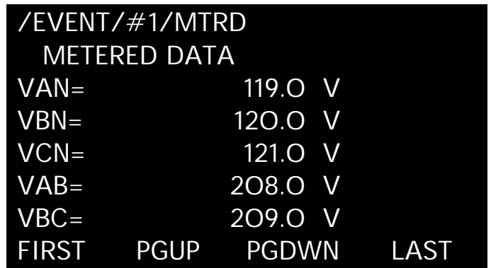
Figure 5-25 Typical Metered Event Voltage Screen
