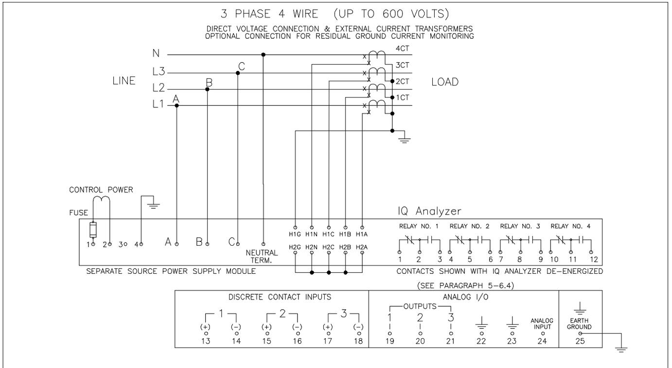
Figure 4-21. 3-phase 4-Wire (Up to 600 Volts) Wiring Diagram
