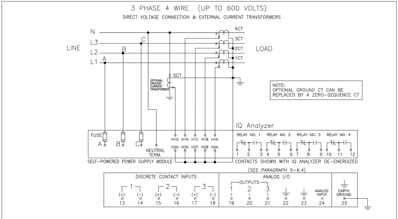
Figure 4-17. 3-phase 4-Wire (96 to 600 Volts) Wiring Diagram
