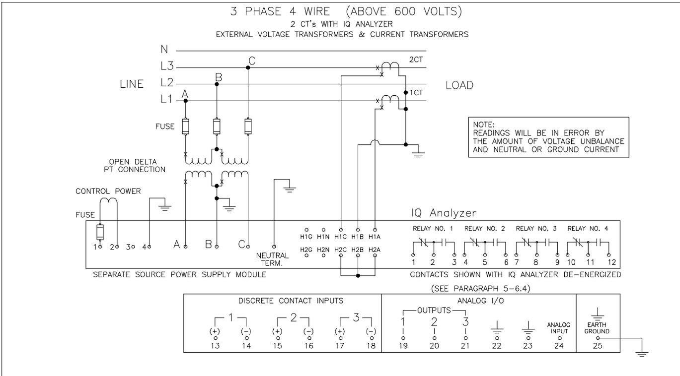
Figure 4-27. 3-phase 4-Wire (Above 600 Volts) Wiring Diagram
