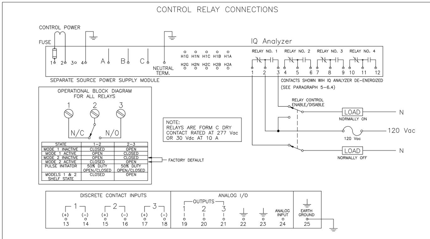
Figure 4-34. Control Relay Connections
