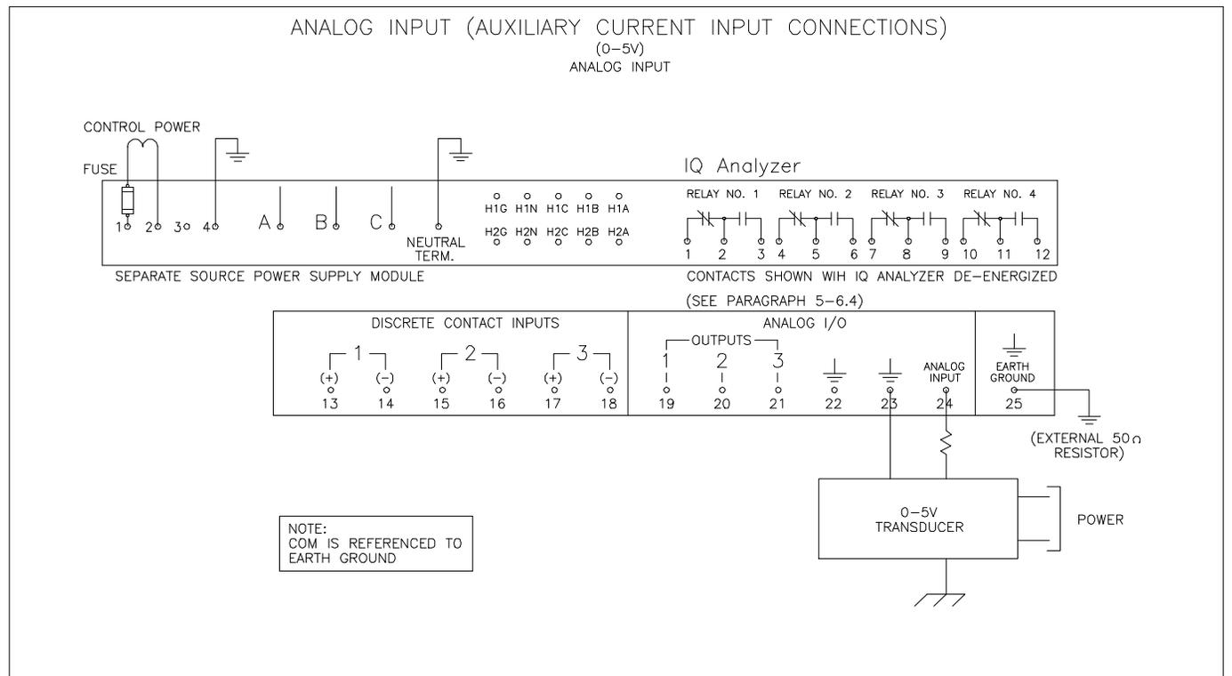
Figure 4-32. Analog Input (Auxiliary Current Input Connections)
