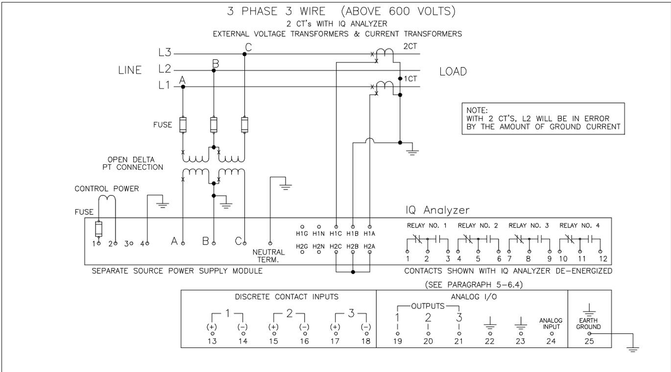
Figure 4-11. 3-phase 3-Wire (Above 600 Volts) Wiring Diagram
