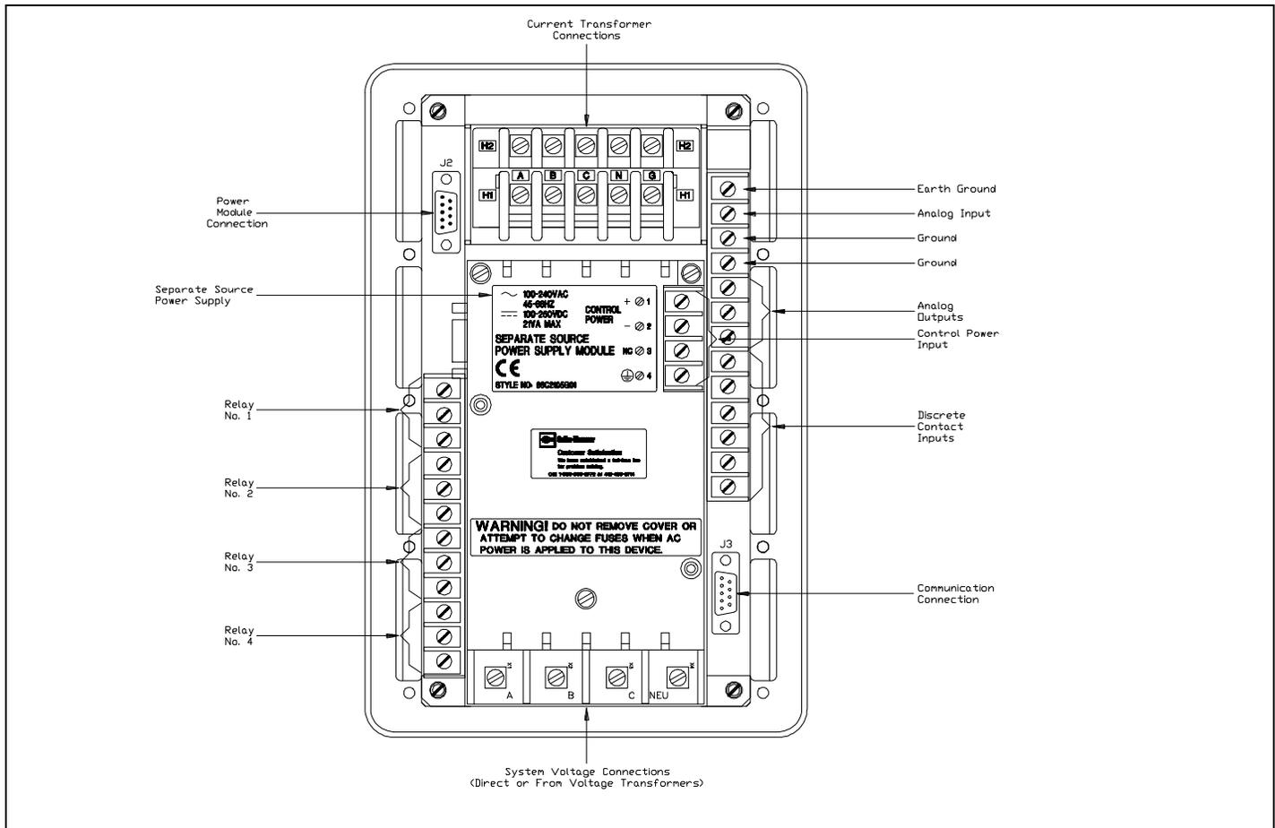
Figure 4-8. IQ Analyzer with Separate Source Power Module (Rear View)
