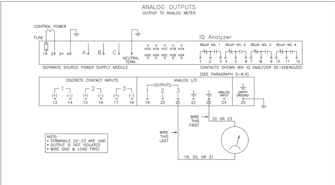
Figure 4-30. Analog Outputs
