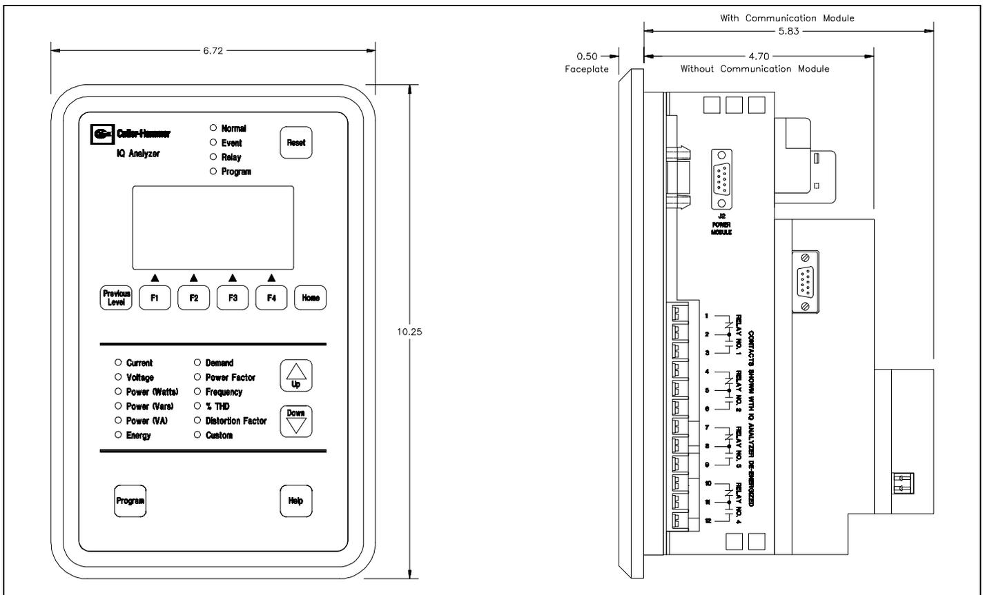
Figure 4-1. IQ Analyzer Dimensions and Cutout (inches)
