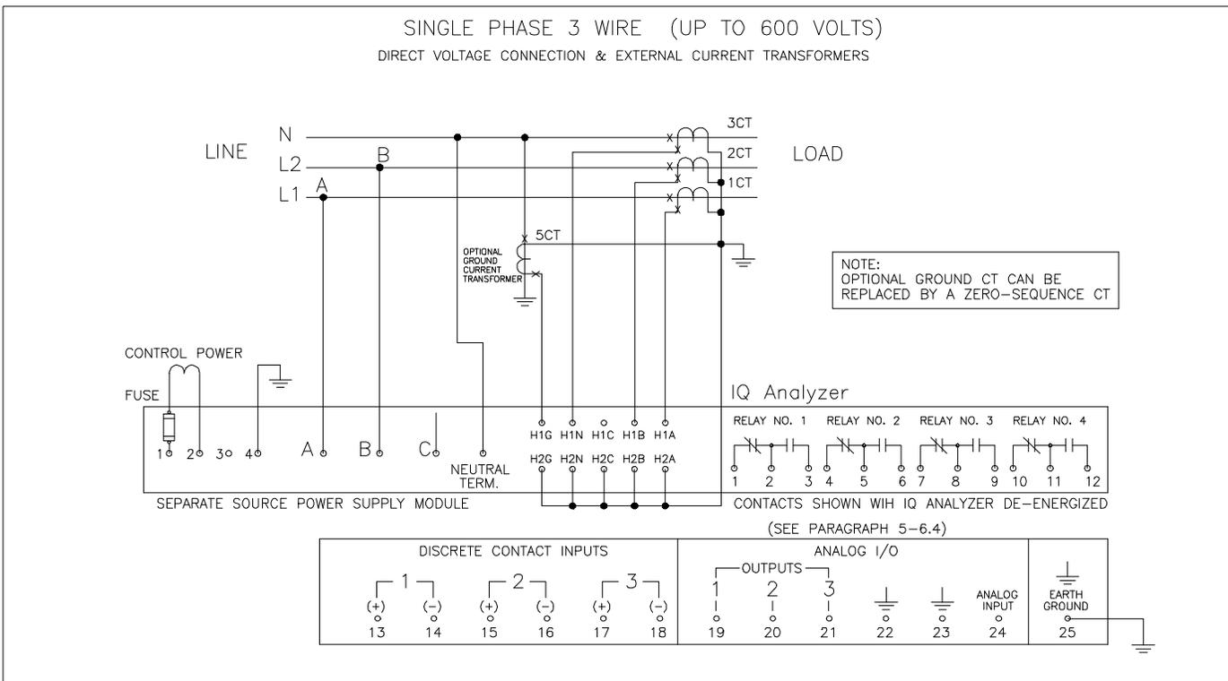
Figure 4-28. Single-phase 3-Wire (Up to 600 Volts) Wiring Diagram
