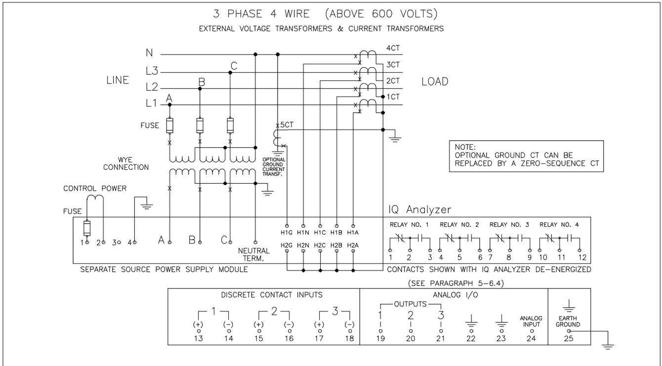
Figure 4-13. 3-phase 4-Wire (Above 600 Volts) Wiring Diagram
