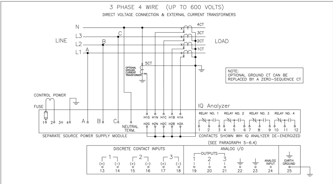
Figure 4-12. 3-phase 4-Wire (Up to 600 Volts) Wiring Diagram
