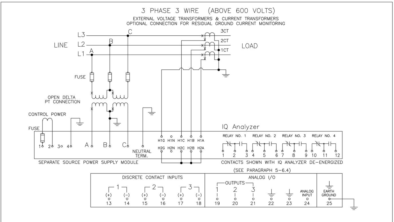
Figure 4-10. 3-phase 3-Wire (Above 600 Volts) Wiring Diagram
