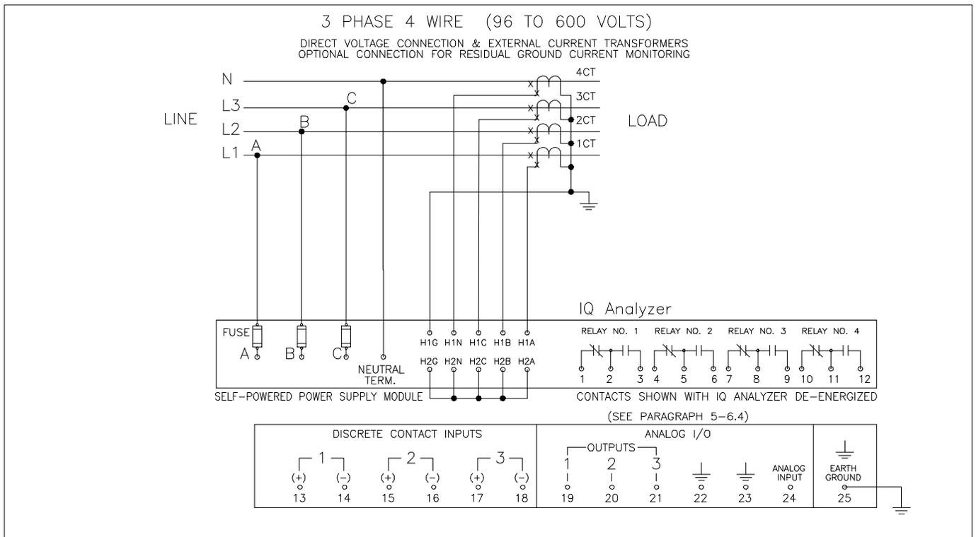
Figure 4-26. 3-phase 4-Wire (96 to 600 Volts) Wiring Diagram
