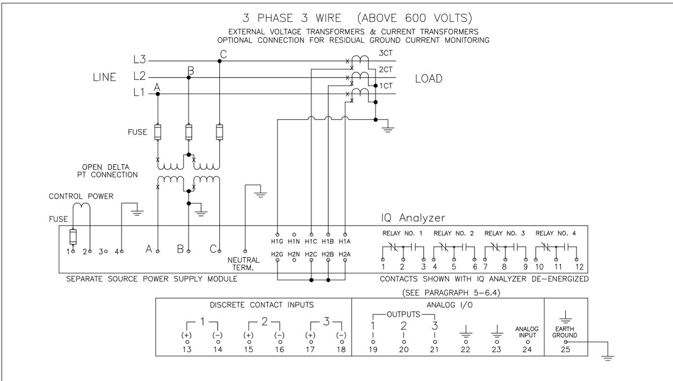
Figure 4-20. 3-phase 3-Wire (Above 600 Volts) Wiring Diagram
