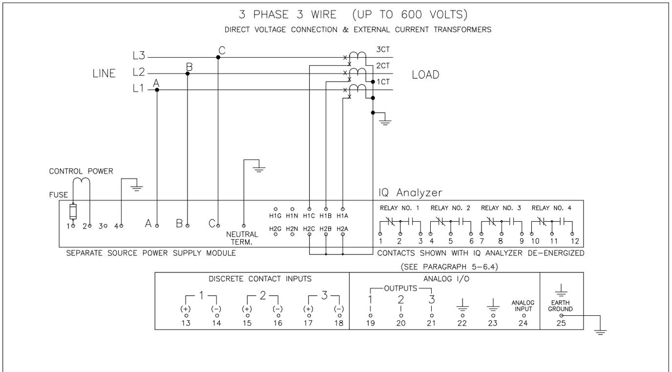
Figure 4-9. 3-phase 3-Wire (Up to 600 Volts) Wiring Diagram
