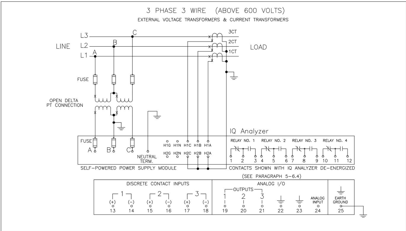
Figure 4-15. 3-phase 3-Wire (Above 600 Volts) Wiring Diagram
