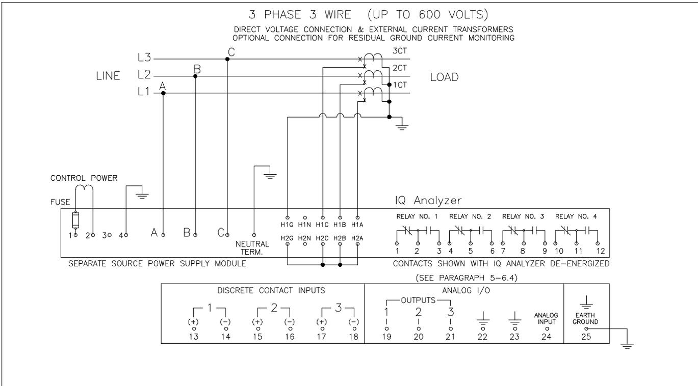
Figure 4-19. 3-phase 3-Wire (Up to 600 Volts) Wiring Diagram
