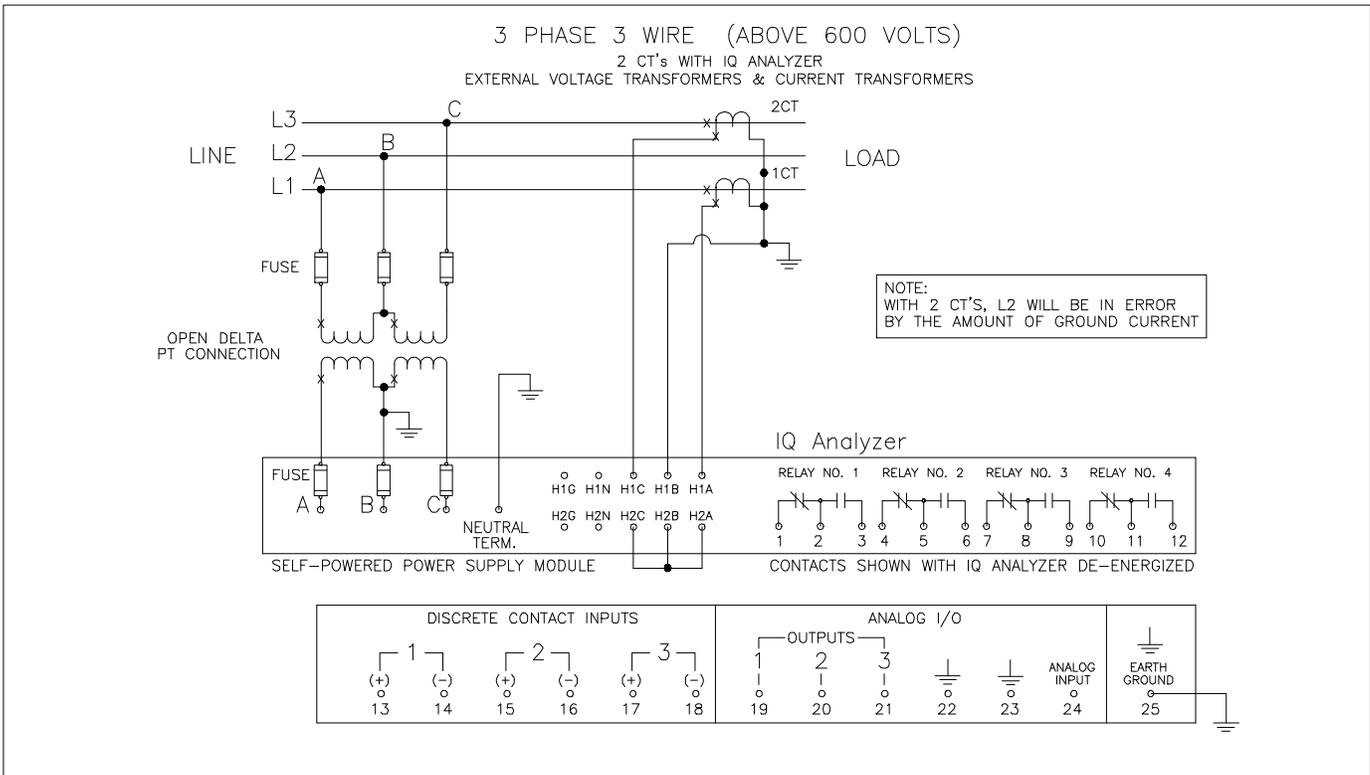
Figure 4-16. 3-phase 3-Wire (Above 600 Volts) Wiring Diagram
