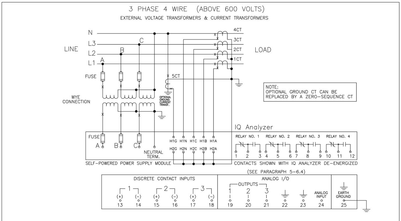
Figure 4-18. 3-phase 4-Wire (Above 600 Volts) Wiring Diagram
