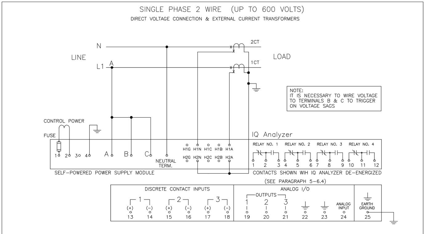
Figure 4-29. Single-phase 2-Wire (Up to 600 Volts) Wiring Diagram
