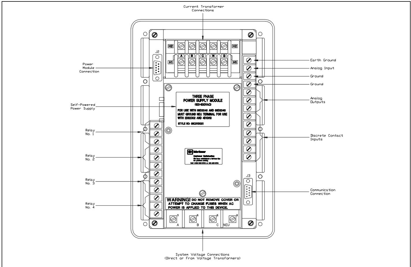
Figure 4-7. IQ Analyzer with Self-Powered Three Phase Power Module (Rear View)
