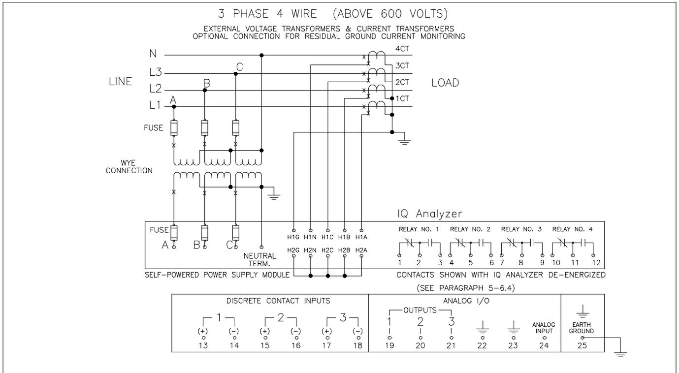
Figure 4-25. 3-phase 4-Wire (Above 600 Volts) Wiring Diagram
