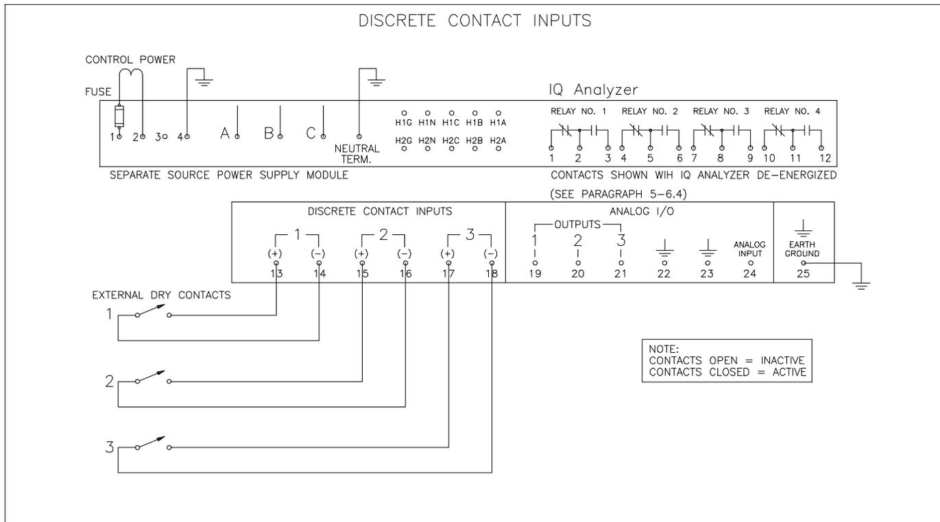
Figure 4-33. Discrete Contact Inputs
