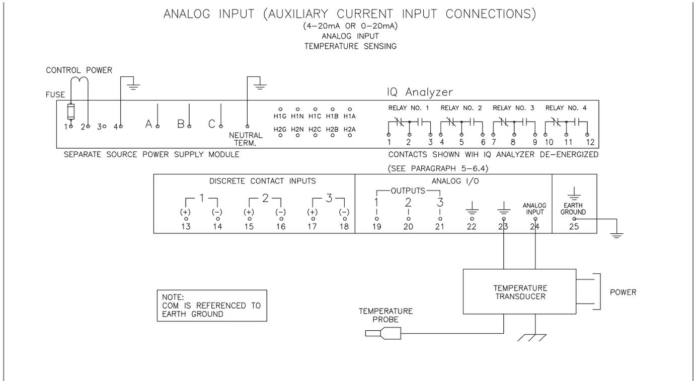
Figure 4-31. Analog Input (Auxiliary Current Input Connections)
