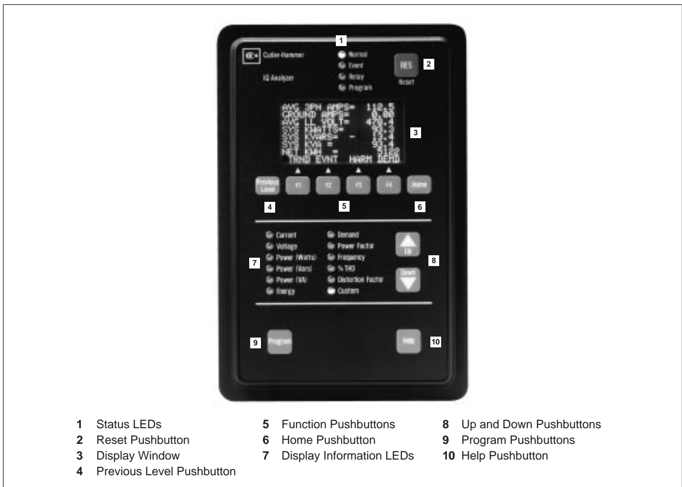
Figure 2-1 IQ Analyzer Operator Panel
