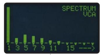
harmonic. The IQ Analyzer also provides a graphical harmonic spectrum bar chart so you can quickly identify the magnitude of each harmonic and pinpoint the source of potentially harmful harmonics.
