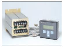
Unique mounting flexibility is provided by the base module (left) which can be display-mounted, panel-mounted, DIN rail-mounted or side-mounted. The display (right) fits into a standard 1/4 DIN cut-out, and for retrofit applications, a 100 mm ANSI collar is available.
