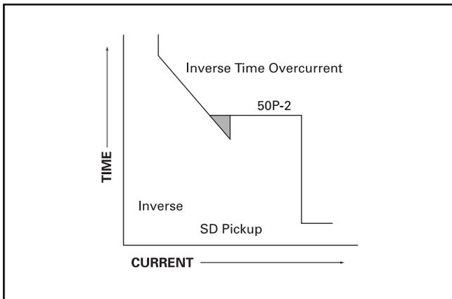
**Figure 8-7. Typical Curve with I<sup>2</sup>t Shape**
