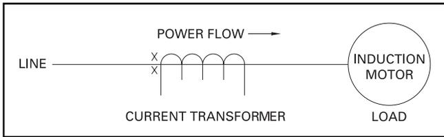
Figure 4-5. Induction Motor Load
