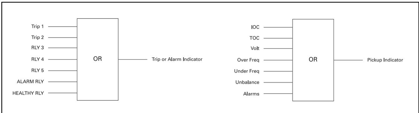
**Figure 9-2. Trip and Alarm Indicator/Pickup Indicator**
