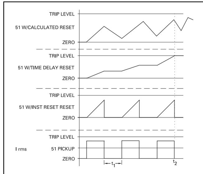
**Figure 5-1. Graphical Representation of the TOC Reset T Setting**
