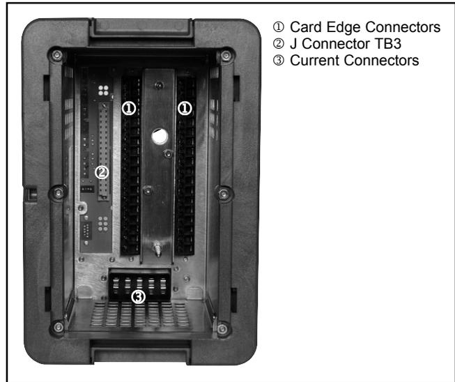
Figure 6-7. Internal View of Case Connectors
