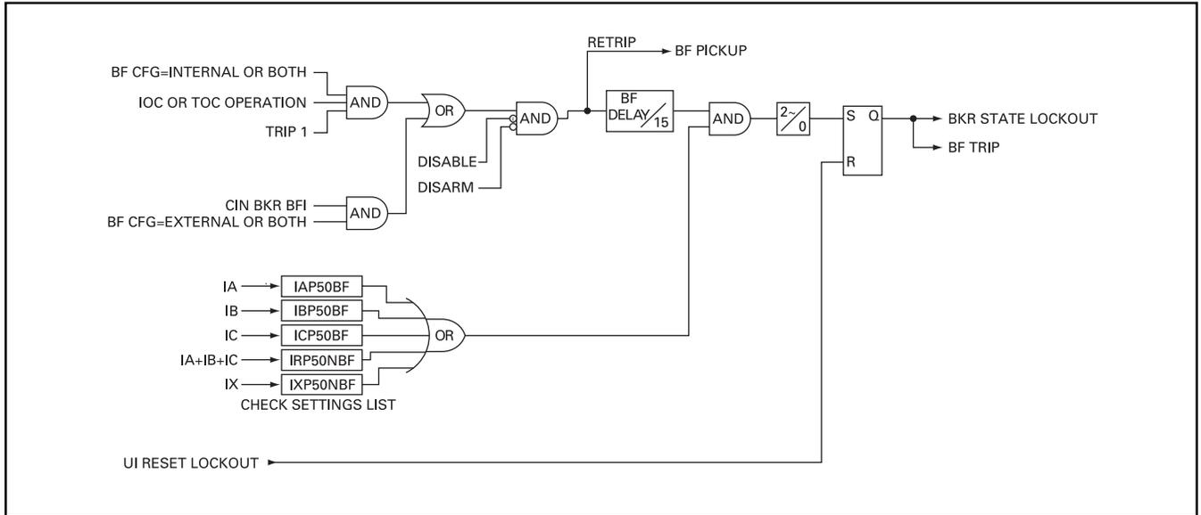
Figure 5-2. Breaker Failure Logic Diagram
