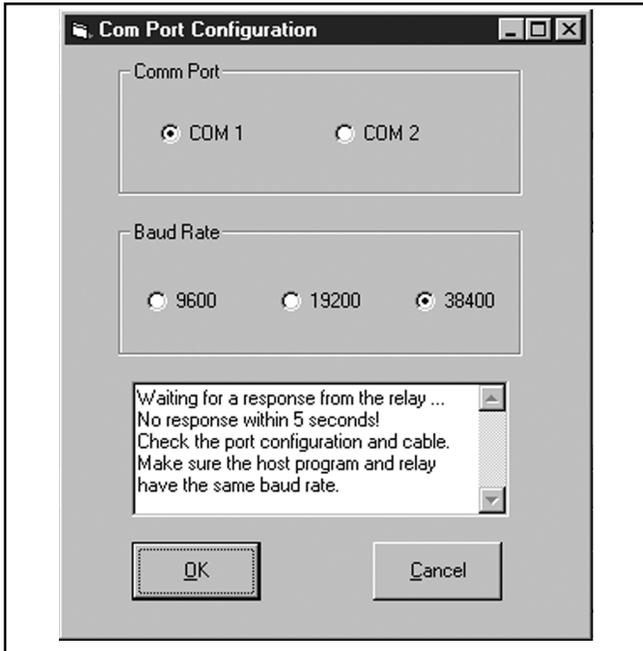
Figure 12-1. Flash Programmer Com Port Configuration
