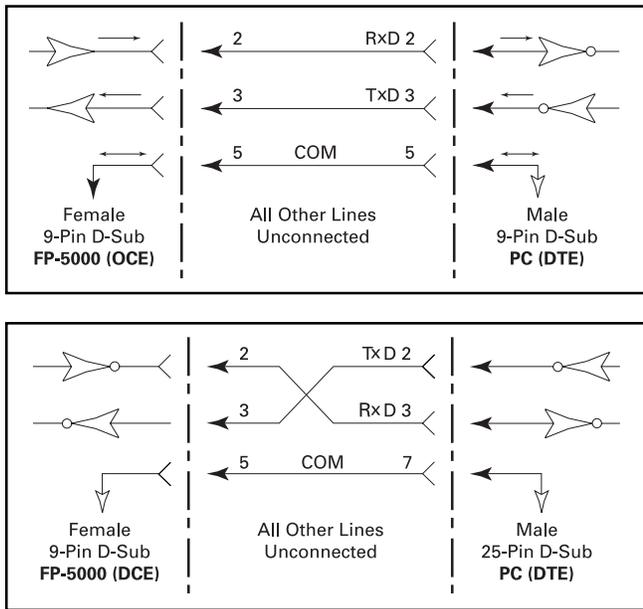
**Figure 4-2. RS-232 Cable for 9- and 25-pin D-Subminiature Connectors**
