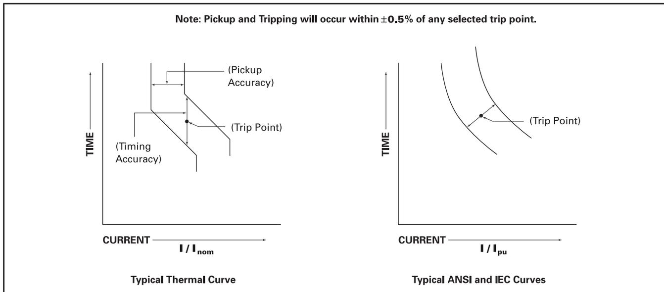
Figure 8-5. Sample Electronic Trip Curves
