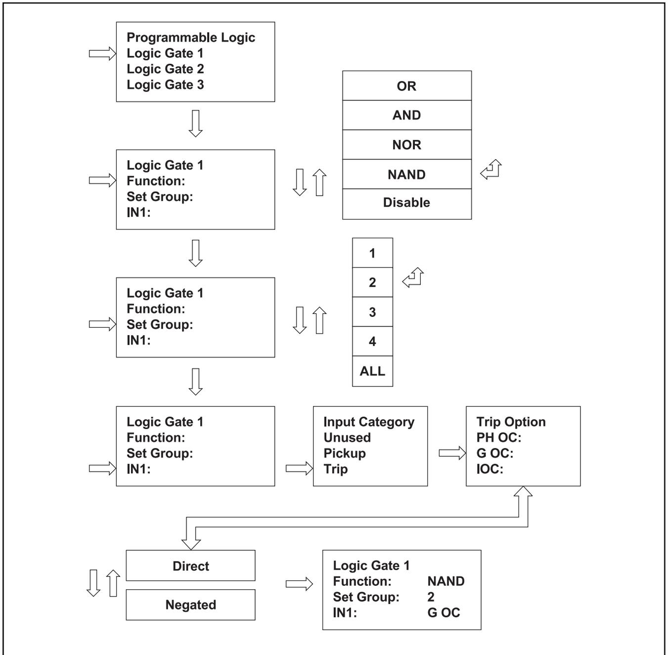
Figure 5-3. Logic Setting Flowchart
