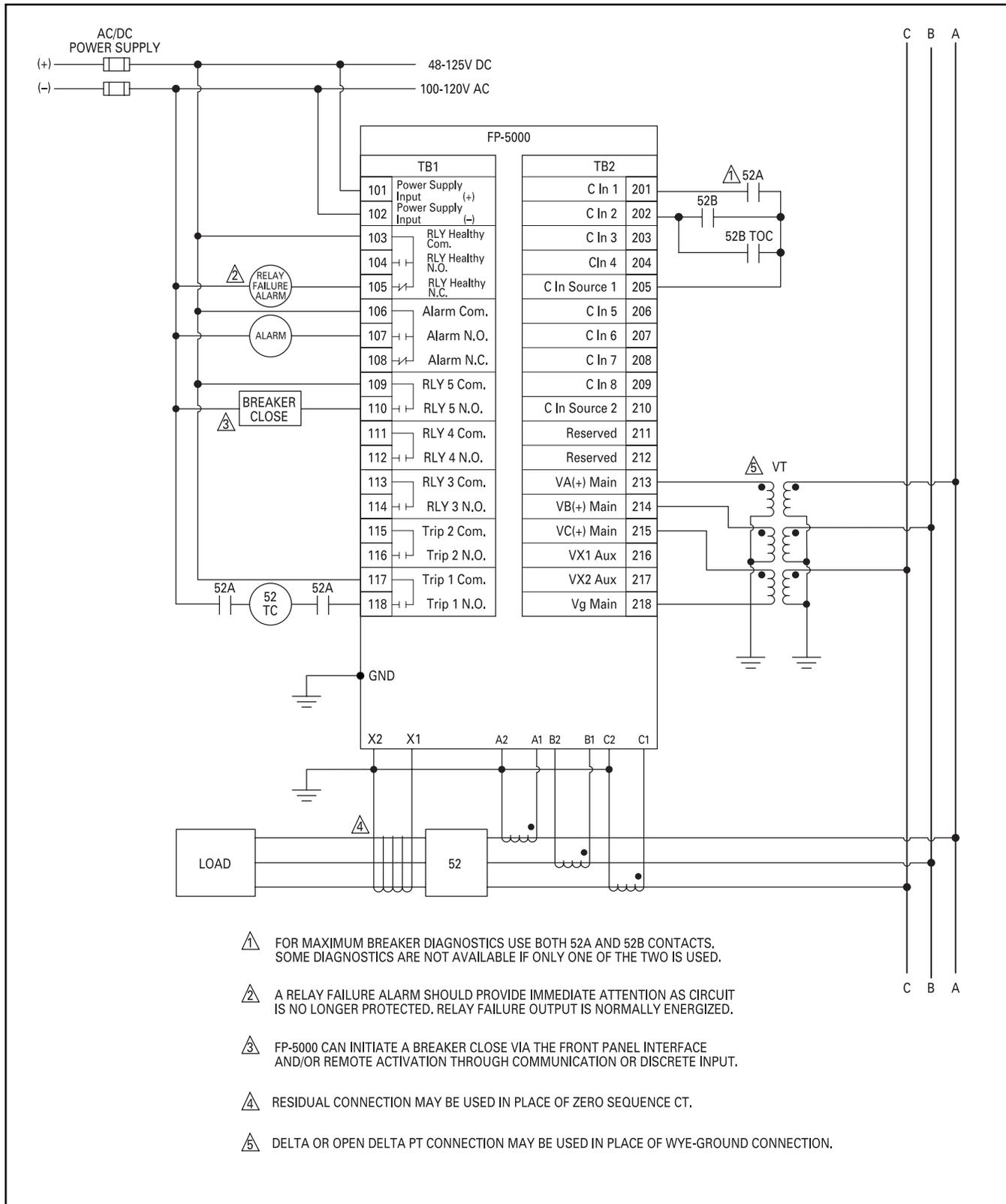
Figure 2-2. FP-5000 Simple Wye Connected Application
