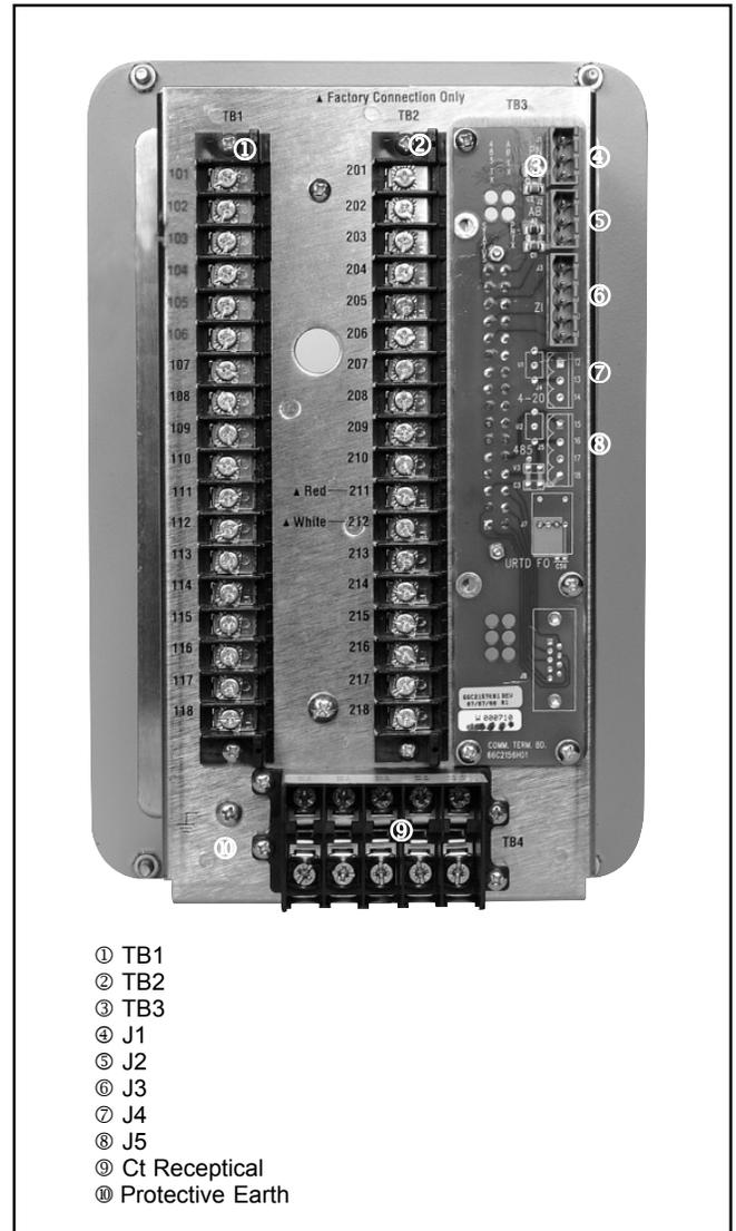
**Figure 6-4. FP-5000 Outer Chassis Rear Connections**
