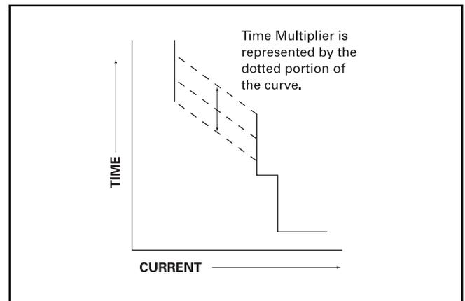
**Figure 8-8. Typical Time Multiplier Adjustment (I<sup>2</sup>t Response)**
