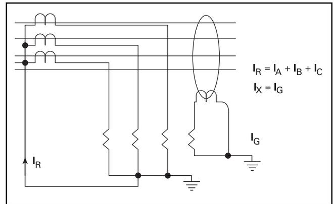
Figure 8-1. Three-Wire Ct Connection
