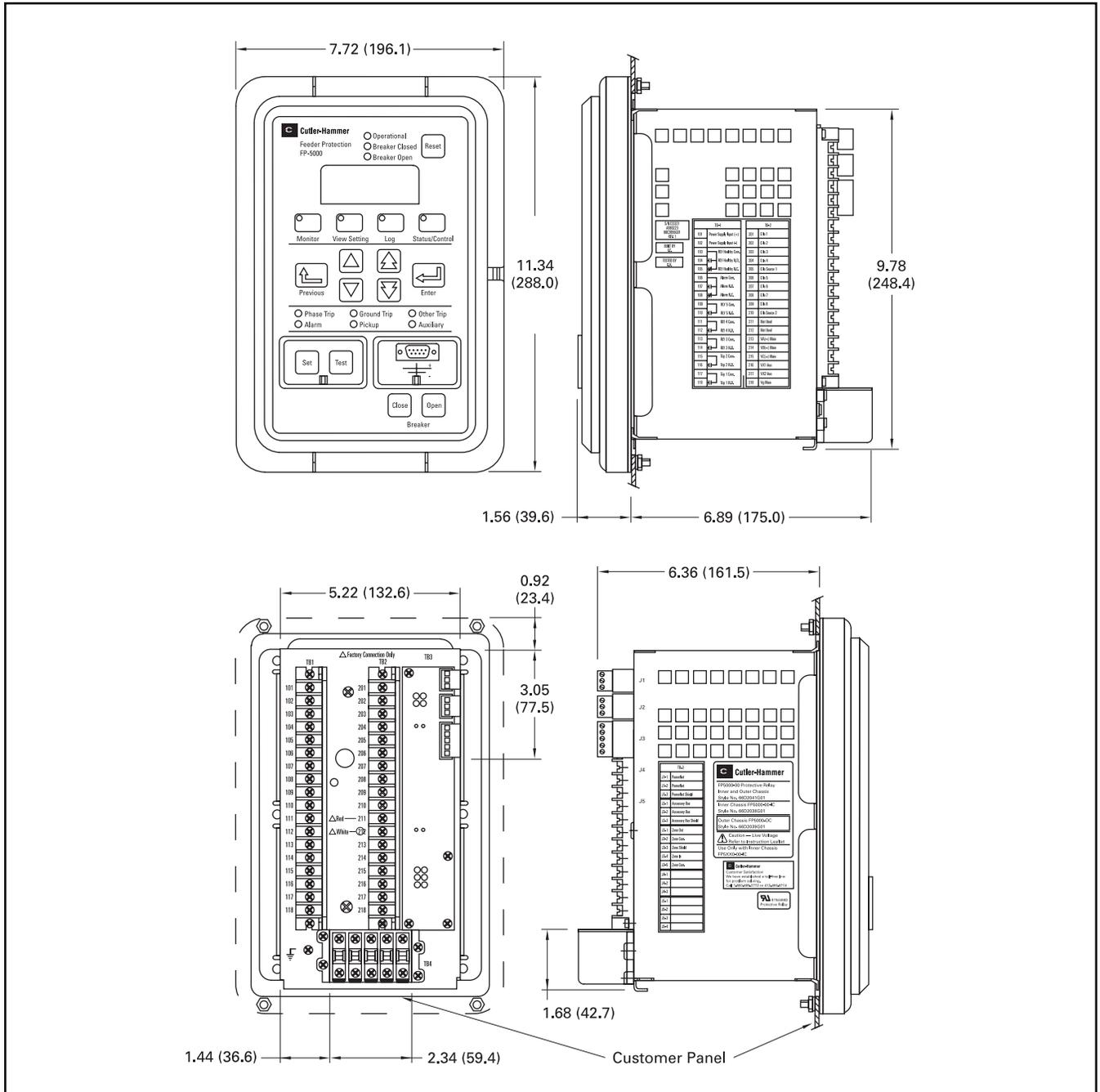
Figure 6-1. Panel Cutout and Mounting Holes
