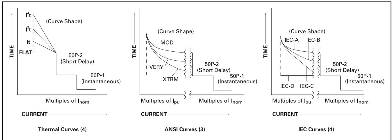
Figure 8-4. FP-5000 Time-Current Characteristic Curves
