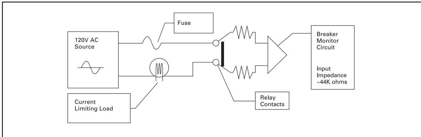
Figure 11-1. Testing Trip Monitors
