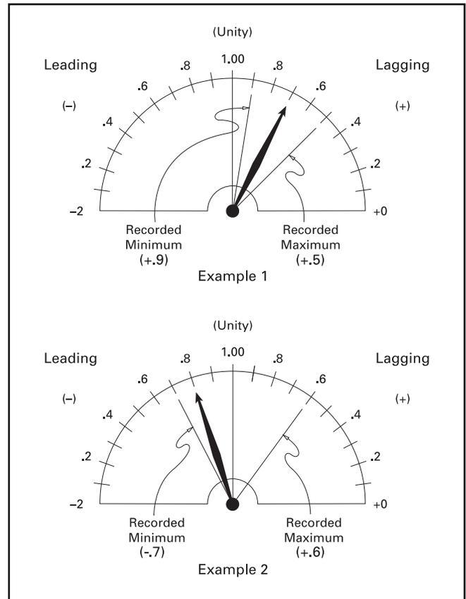
Figure 4-3. Power Factor Minimum/Maximum
