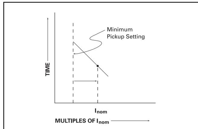
Figure 8-6. Typical Inverse Time Overcurrent Pickup Horizontal Movement
