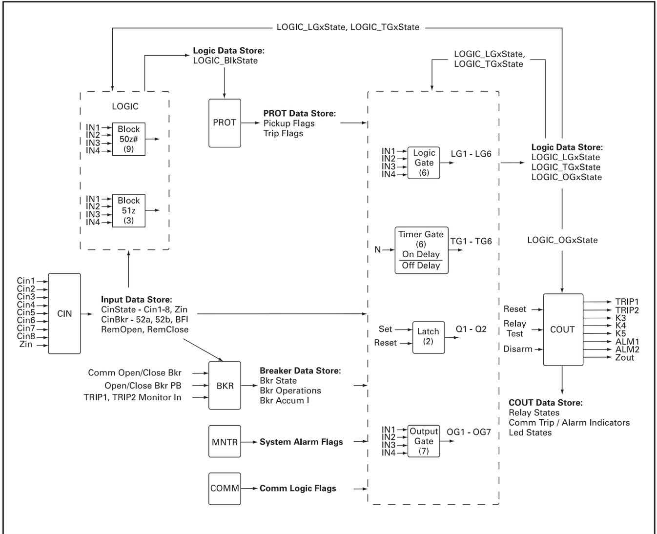
Figure 9-1. Overall Logic Diagram
