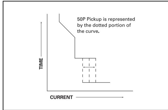
**Figure 8-9. 50P (Instantaneous) Setting Adjustment**
