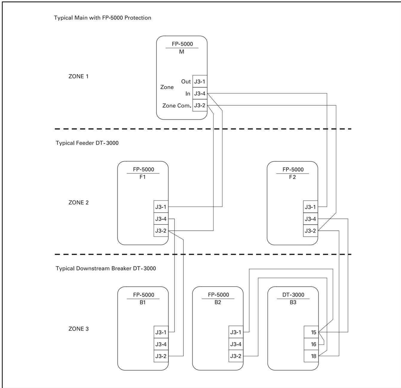
**Figure 8-10. Zone Interlocking Example with FP-5000 and DT-3000**
