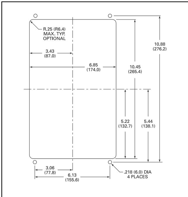
**Figure 6-2. Panel Cutout and Mounting Holes**
