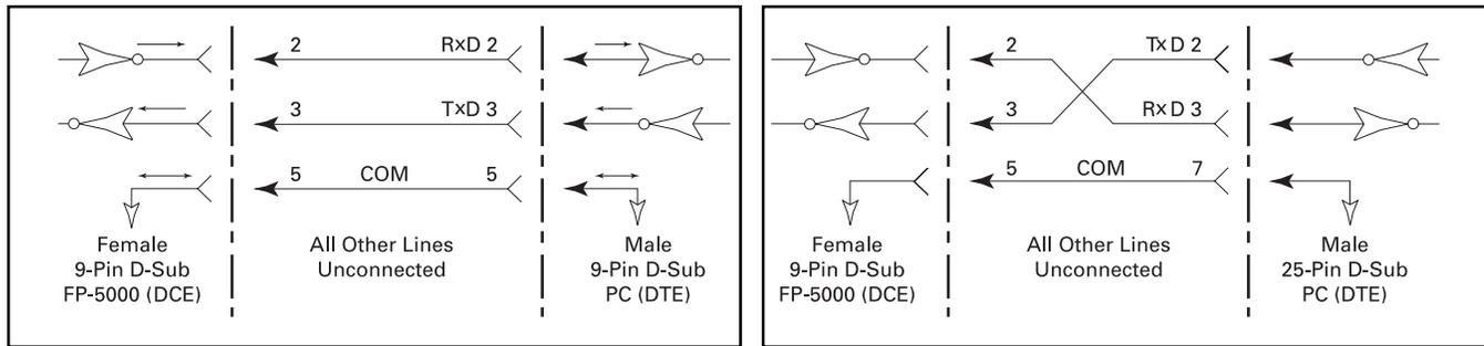
Figure 10-2. RS-232 Cable for 9- and 25-pin D-Subminiature Connectors
