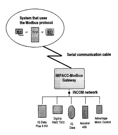
The following diagram shows a detailed example of communication between the Modbus Gateway and devices.
