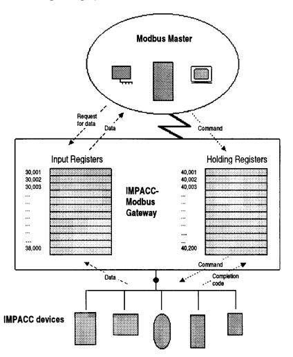
The Modbus Master sends a command intended for a particular device. For example, it might send the command "0x600" to device #102.
