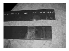
Figure 2 Corona detected and damage found between cubicles # 8-9
