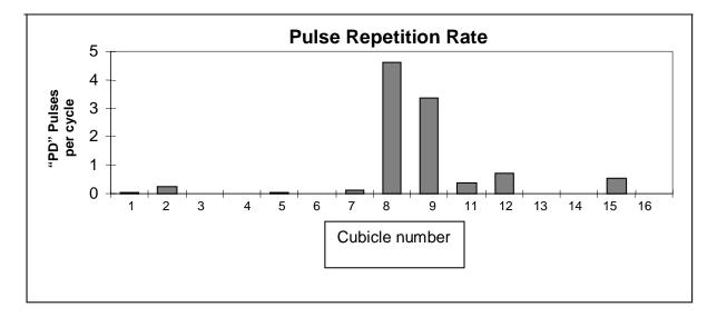
Figure 1 On-Line Partial Discharge Detection in medium voltage switchgear
