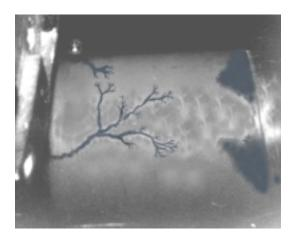
Figure 3 Surface Tracking on a 4160-Volt Circuit Breaker Bushing
