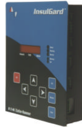
Continuous Partial Discharge Monitor
